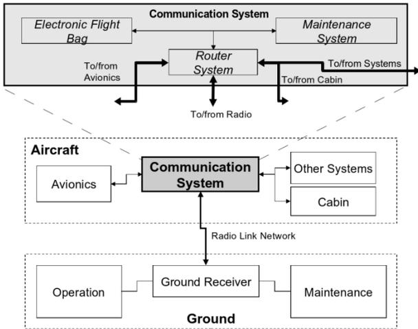
Figure 2: System level and extended system context with three dedicated system elements
