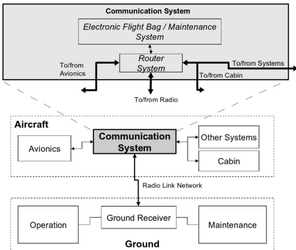
Figure 3: System level and extended system context with two dedicated system elements
