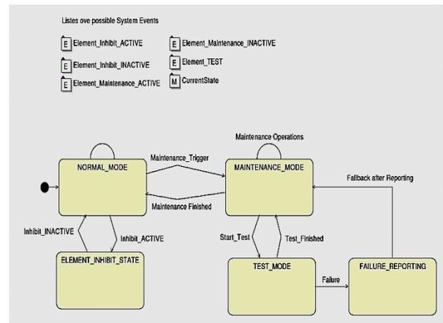
Figure 8: Possible slave states of the Normal state of an Element FSM
