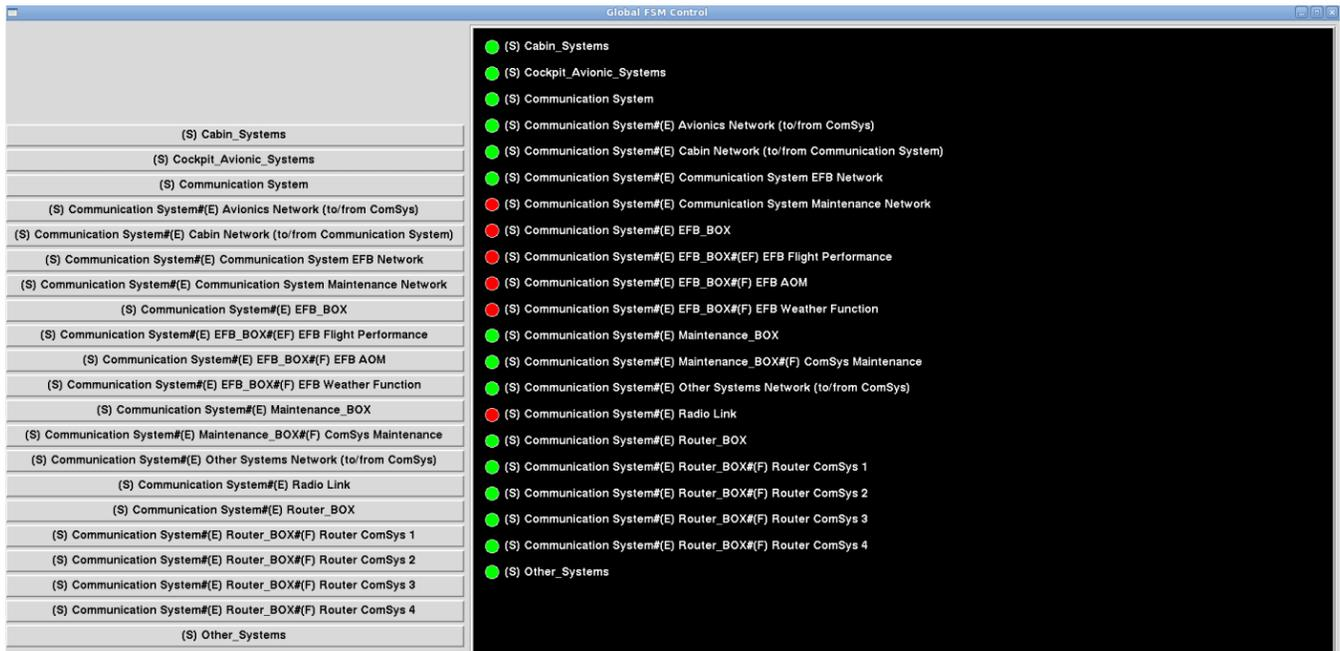
Figure 10: Automatically created GUI to observe (right hand side) and control (left hand side) the execution of different systems, Elements and Functions during simulation of the communication system
