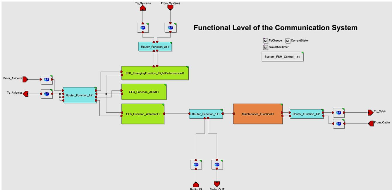
Figure 4: Functional blocks of the communication system on system level in MLDesigner
