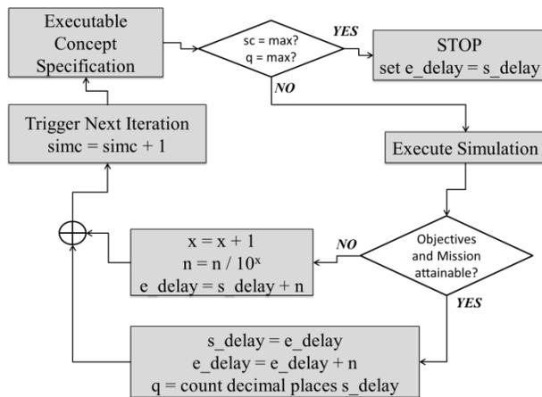
Figure 9: Sequence plan for maximum valid Element delay calculation through iteration with MLDesigner
