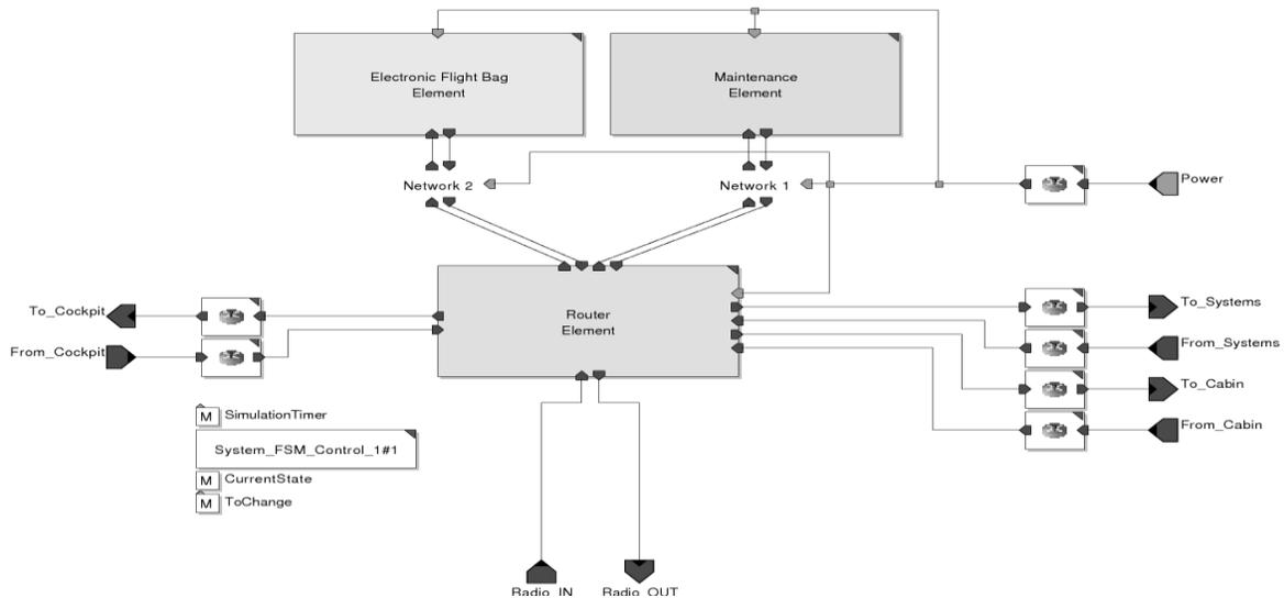
Figure 7: Variant 1 of the communication systems conceptual architecture in MLDesigner containing 3 ECUs and 2 network Elements
