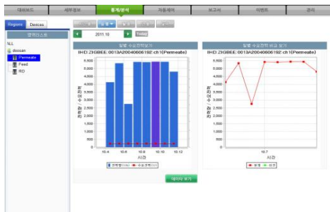
Figure 5. Measured Power Usage Data from Small Size Desalination Plant
