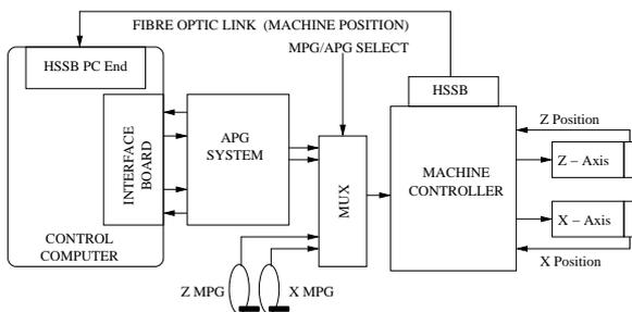
Figure 1: Schematic of the external axis control system
