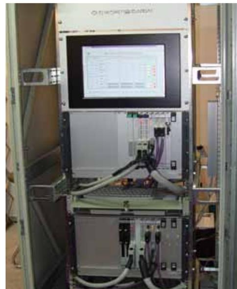
Figure 6. Front Panel of DRPS Prototype
