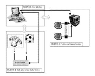
The LoT data acquisition system is based on a triaxial accelerometer, embedded in a ball, and on a variable number of modules (namely, the SensVest modules) embedded in a simple wearable, a shirt. Each SensVest hosts bi-axial accelerometric sensors for tracing of body, arm and leg accelerations, and two other sensors for reading of temperature and heart rate physiological parameters<sup>2</sup>.
