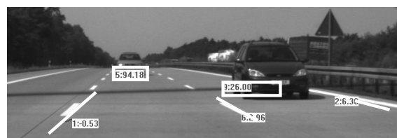
Fig. 21. Lane Detection with the Hough Transform
