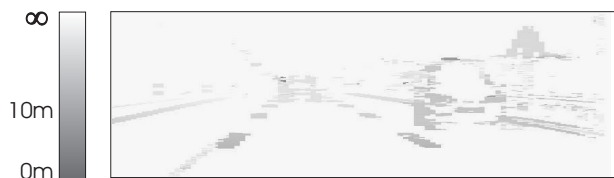
Fig. 11. Generated depth map (distance coded with gray values)
