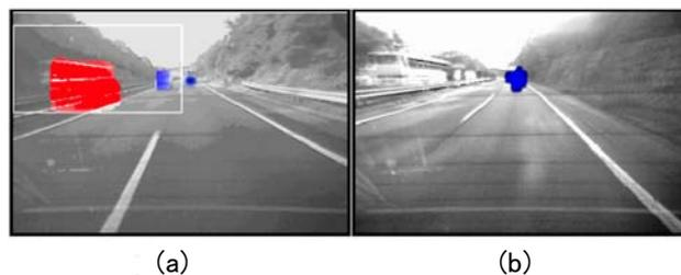
Fig.9 Illustration of the comparison between the MLP-based and RNN-based detection methods. (a)Detection result with the MLP (conventional) method. (b)Detection result with the RNN (suggested) method.
