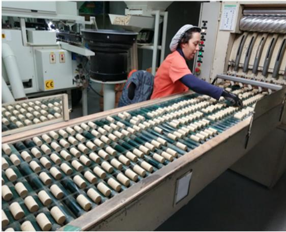
Fig. 7. Manual picking process.
