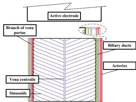
Fig. 3. Simplified geometric model of hepatic tissue in 2D setup
