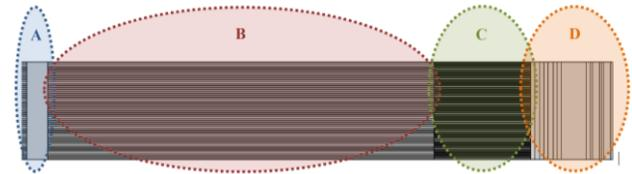
Fig. 4. 2D – Axisymmetric simulation model of hepatic lobule respecting the electrical heterogeneity of tissue. Width of excision is 1,2 mm; height is 0,24 mm.
