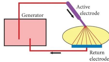
Fig. 2. Principle of configuration for monopolar cutting
