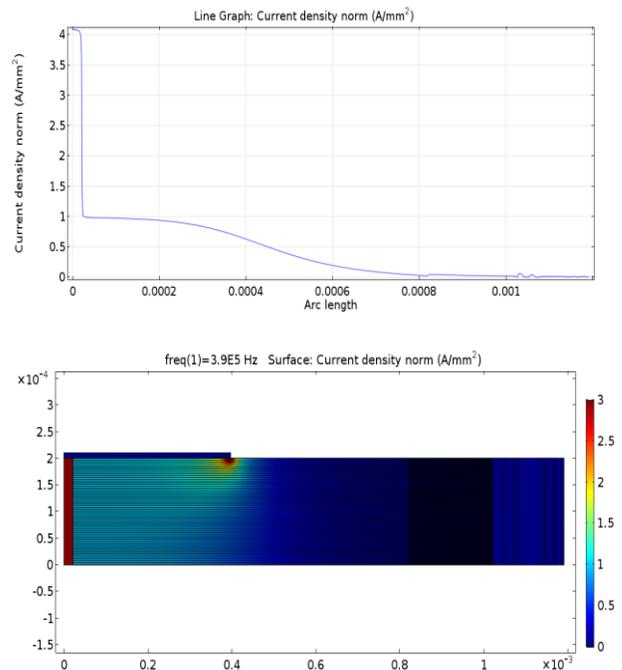
Fig. 6. Current density distribution (top) and streamline current density (bottom) in liver tissue at  $d=0$  mm, heterogenous complex simulation model
