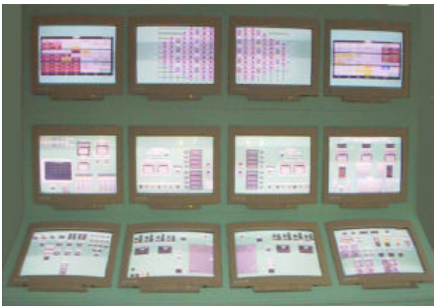
Figure 4. Prototype built to accommodate twelve soft panels.
