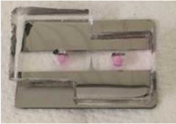
Fig. 5: Flow channel with surface electrodes. 10 mm
