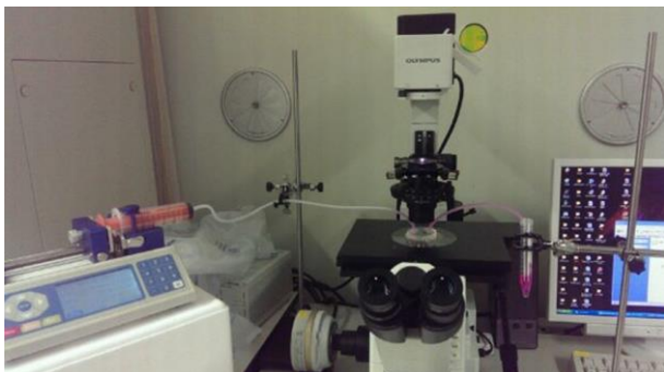
Fig. 2: Flow test system: flow chamber and microscope (middle), syringe pump (left).
