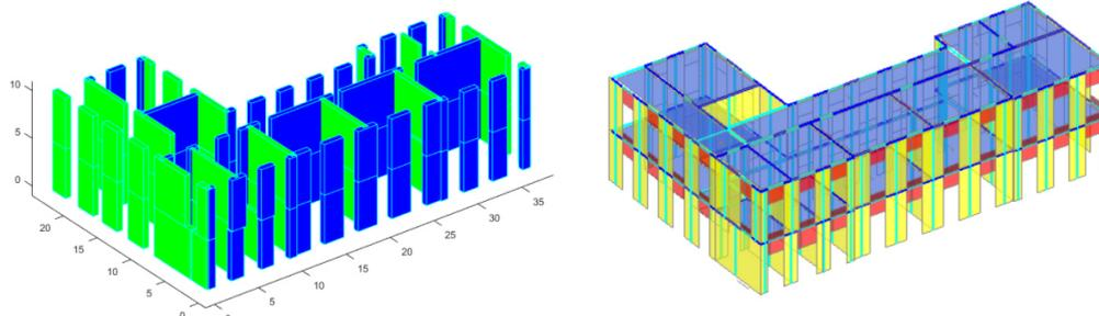
Fig. 5. 3D-Layout of the resistant shear walls (E-PUSH) and equivalent frame model in Aedes PCM
