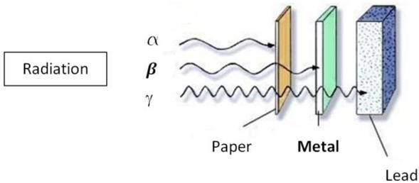
Figure 3: Radiation types and blocking materials
