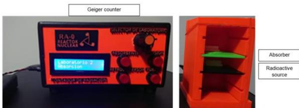
Figure 5: Simulated absorption experiment setup
