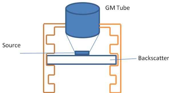
Figure 8: Backscattering experiment schematic setup
