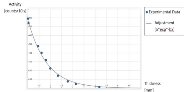
Figure 6: Simulated absorption experiment curve fitting
