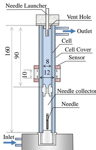
Fig.2 Schematic diagram of the compact-sized falling needle rheometer for measurement of blood viscosity
