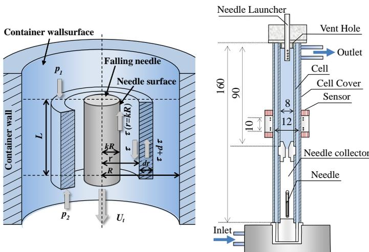
Fig.1 Flow model of the sample fluid in the fluid vessel of falling needle rheometer
