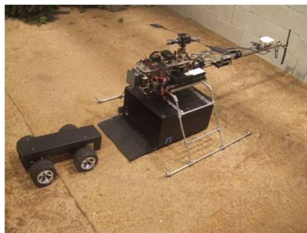
Figure 1. A belly-mounted docking station permits the robotic helicopter to aerially transport an unmanned ground vehicle
