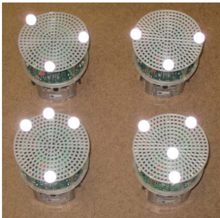
Figure 7: Optical Tracking Reflectors on E-puck Robots.
