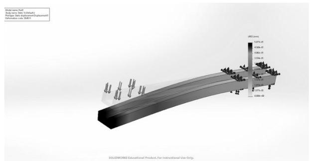
Figure 8 (top): Beam with load, photo by Steinar Killi; Figure 9 (middle): CAD drawing of beam with loads and boundary conditions, screenshot by Steinar Killi; Figure 10 (bottom): Simulation of Beam with load, screenshot by Steinar Killi.
