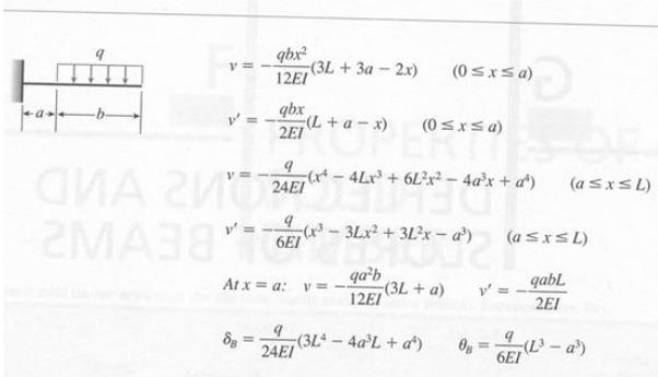
Figure 6 (top): The plastic beam, photo by Steinar Killi; Figure 7 (bottom): Formulas for load on a beam.
