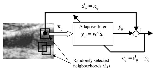
Fig. 2. The adaptive process
