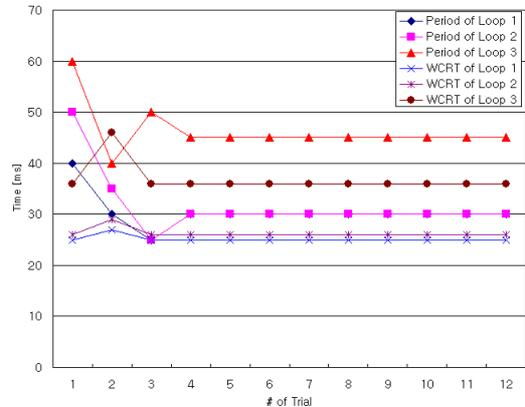
Fig.6 CAN: 100kpbs under no noise condition
