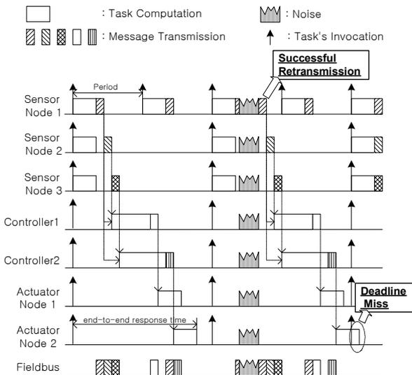
Fig.1 End-to-end response time delayed by noise
