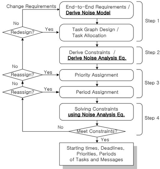
Fig.3 Task and message scheduling under noise environment
