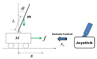
Fig. 1.Teleoperation of an inverted pendulum system
