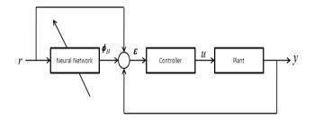
Fig. 4 RCT neural network control block diagram
