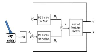
Fig. 2 PID control structure
