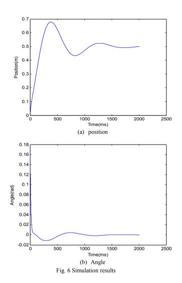
pendulum system is required to move to 0.5 m while balancing. Fig. 6 shows the simulation results. We see that the balancing angle and the cart position are well regulated.
