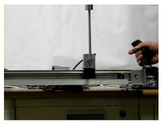
Fig. 10 Joystick command control for inverted pendulum
