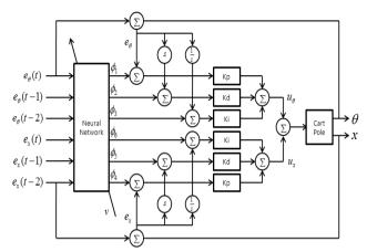
Fig. 5. Neural network control structure
