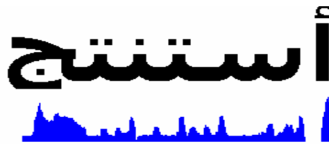
Fig.6 Vertical projection profile of a word
