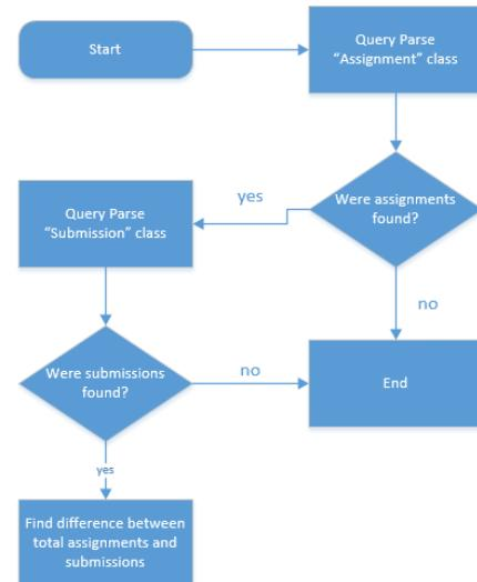
Fig. 3.5: The `getNewAssignment` Algorithm.
