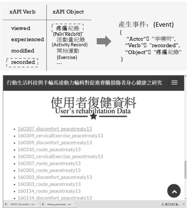
Fig. 9. Users' habits are represented as records in xAPI format. These records are stored in the database and can be studied through the Web.
