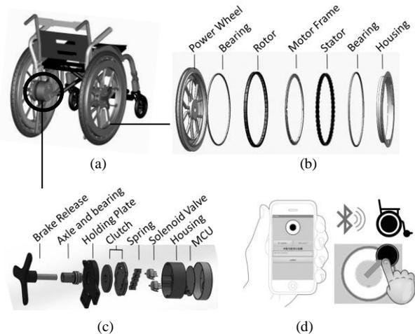
Fig. 2. (a) Configuration of the smart wheelchair driven by dual power wheels, (b) rim motor in the power wheel and its components, (c) brake assembly, and (d) remote control on the smart phone.
