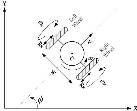
Fig. 3. Skeleton of the wheelchair driven by rim motors.
