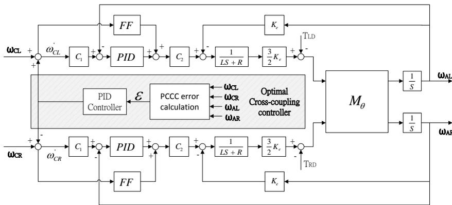
Fig. 4. Optimal cross-coupling control structure.
