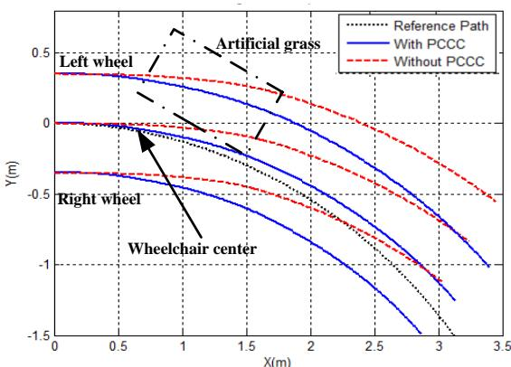
Fig. 7. Trajectories of the left and right wheels before and after the wheelchair drives through the artificial grass with and without the proposed cross-coupling control.
