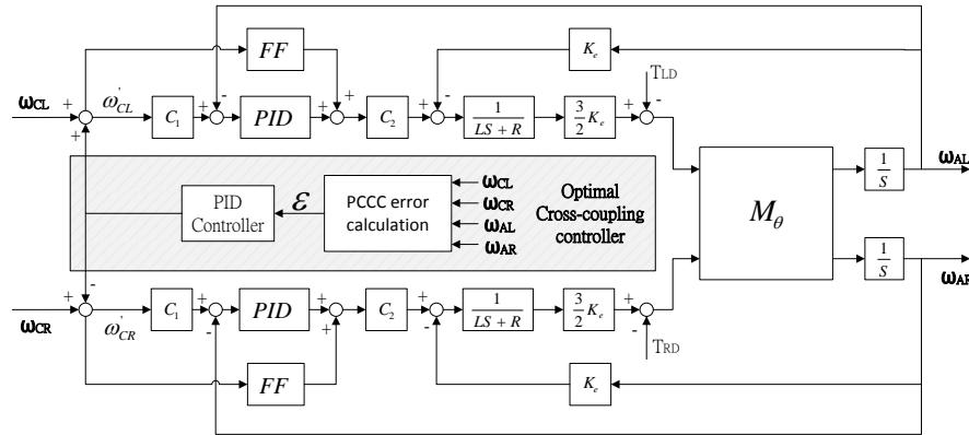
Fig. 4. Optimal cross-coupling control structure.
