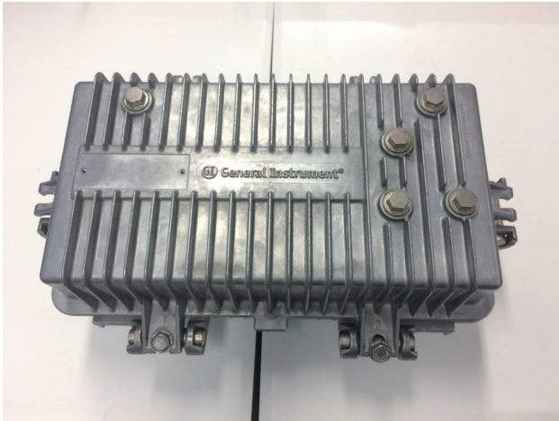
Fig. 7. Overview of inline amplifier.
