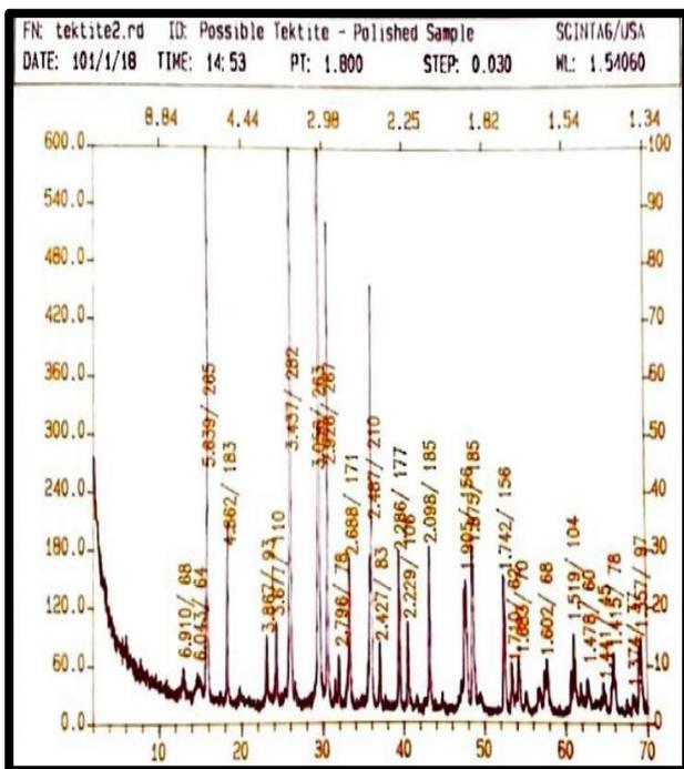
Table 1: X-ray diffraction results of polished sample (Fig. 5) [2].
