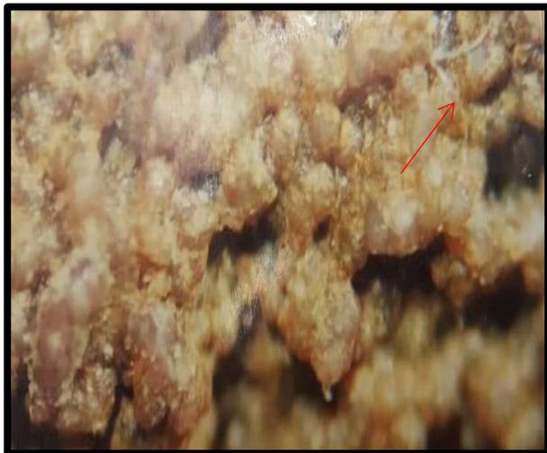
Figure 6: 10x Magnification showing “rounded” grains of glass and filaments in the top right corner.
