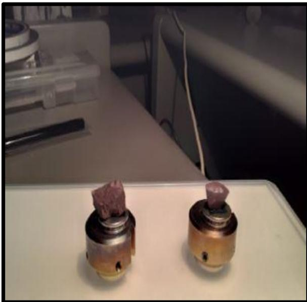
Figure 15: Analcime Scanning Electron Microscopy (SEM) samples. Purple analcime (left) and brown analcime (right).
