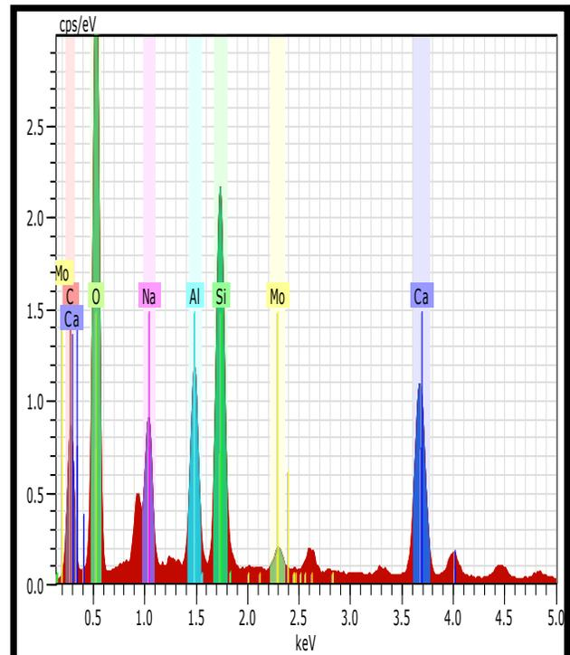
Table 4: Electron Dispersive X-ray Spectroscopy (EDS) of brown analcime sample.
