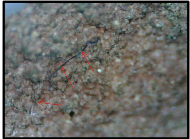
**Figure 9: Image of Filament** at 4x magnification. Here one starts to see how the filament is woven into the isotropic grains. Another filament appears on the bottom of pic or could be the same one.
