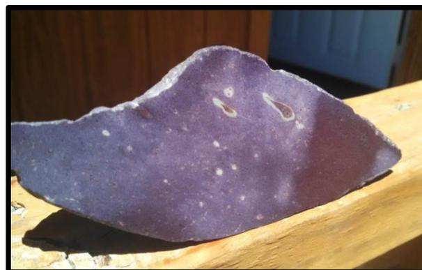
Figure 5: Polished Sample of Obsession Stone used in X-ray Diffraction [2].
