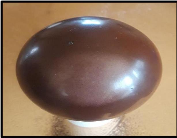
**Figure 7: Round Sample of Obsession Stone** used in X-ray Diffraction [2].
