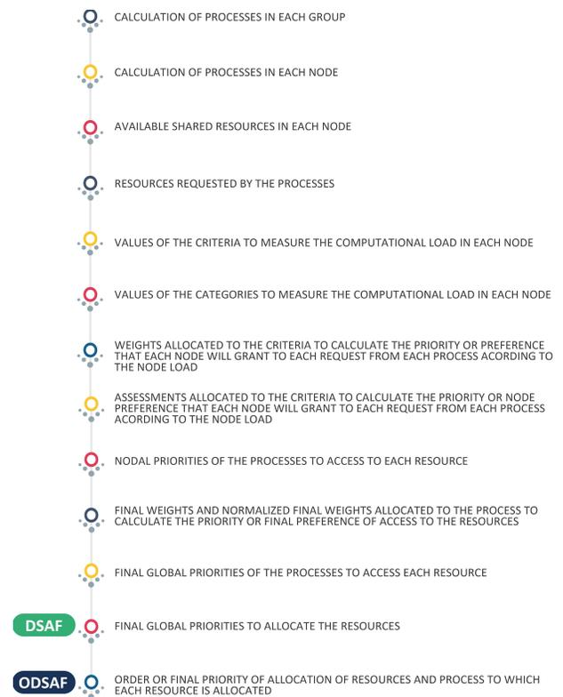
Fig. 2. Steps to obtain the **DSAF** and **ODSAF** functions.
