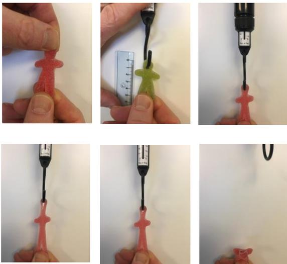
Figure 4 – Using a jelly man, a ruler and a scale to determine Young's modulus and the strength of jelly material. Picture Steinar Killi.
