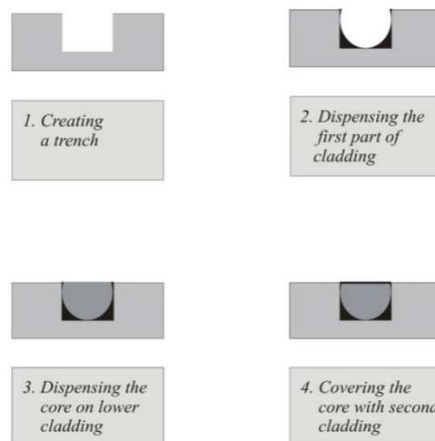
Fig. 2. Production steps for surface integrated dispensed POF
