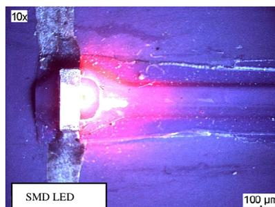
Fig. 3. Directly connected SMD-LED using micro dispensing
