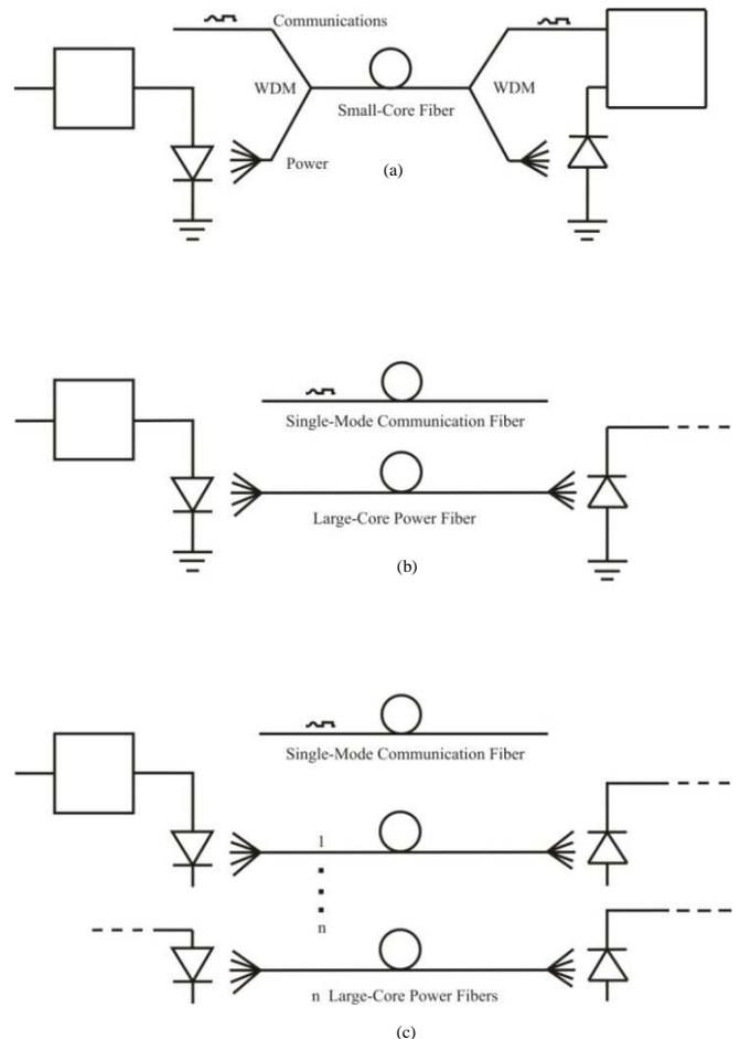
Fig. 1. Powering Architectures. a) Power and data multiplexed on a small-core communications fiber by WDM. b) Separate (single) power fiber. c) Multiple power fibers.
